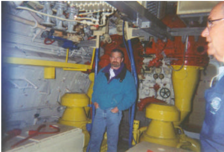
Engine Room looking aft (STBD) – 3 engines abreast. Big one in the middle... 2 smaller ones port and starboard. The square units at Joe’s knee height are Valve Covers. Air to engines coming down from overhead in a turbine-like scoop. “Joe” is Joe Sciola, a neighbor of Bob Culley.
